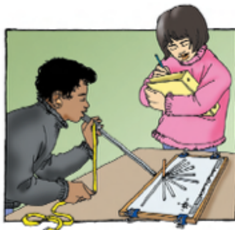
Figure 5.6: Measure the height of the Mini Maglite® at each of the nine points.
