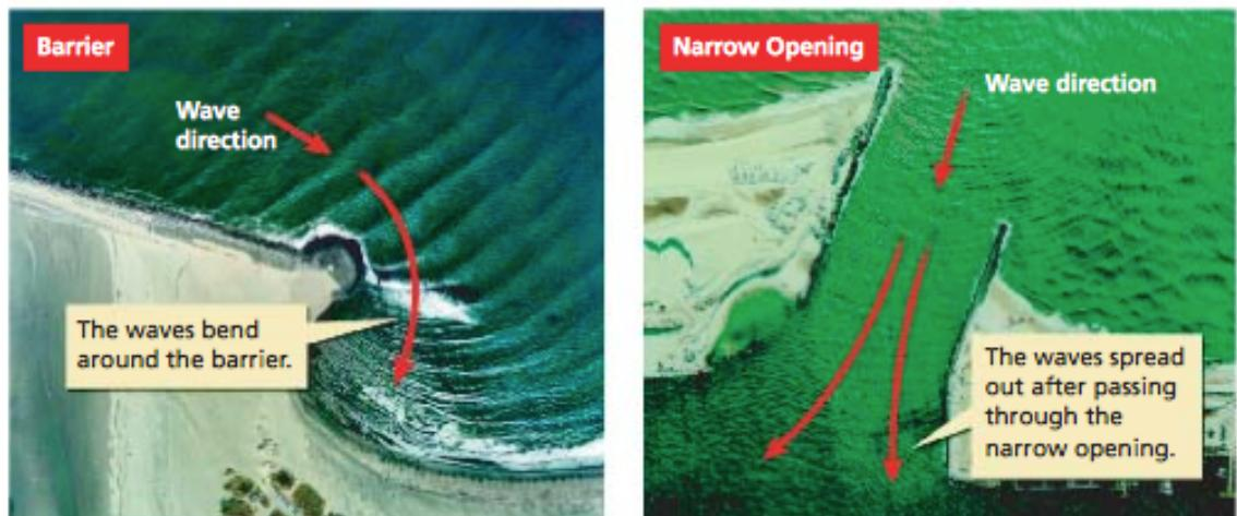
**When a wave passes a barrier or moves through a hole in a barrier, it bends and spreads out.** The bending of waves around the edge of a barrier is known as **diffraction**. The picture above shows a water wave passing through a hole in a barrier and another bending around a barrier. In each case, you see the wave diffracting on the other side of the barrier.
